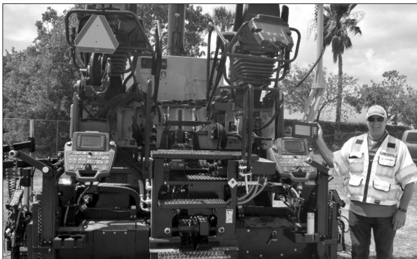
**Brian Girouard, SITECH sales/application engineer from North Las Vegas, spoke with contractors about this Caterpillar AP 500 paver and the Trimble Paving Control System that helps speed up paving production while laying a smoother surface and reducing material costs.**
